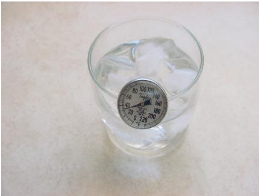
Ice method for calibration of Metal Stem Thermometer
